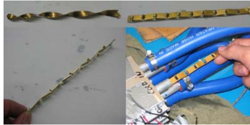
Figure 3. Flow impeding inserts
