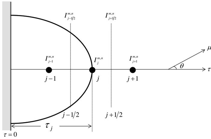
Figure 2: Schematic representation of a pulsed collimated radiation beam propagating in a participating medium.
