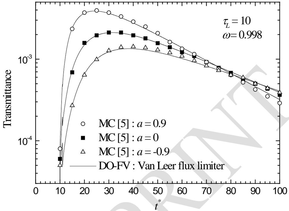
Figure 4: Temporal distribution of the hemispherical transmittance; comparison between the Van Leer flux limiter and a Monte Carlo formulation [5].
