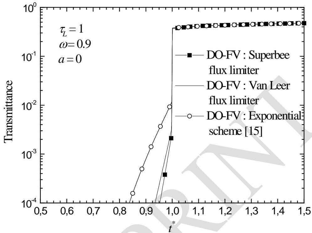
Figure 9: Temporal distribution of the hemispherical transmittance; comparison between the Van Leer and Superbee flux limiters and the exponential interpolation scheme at early time periods.
