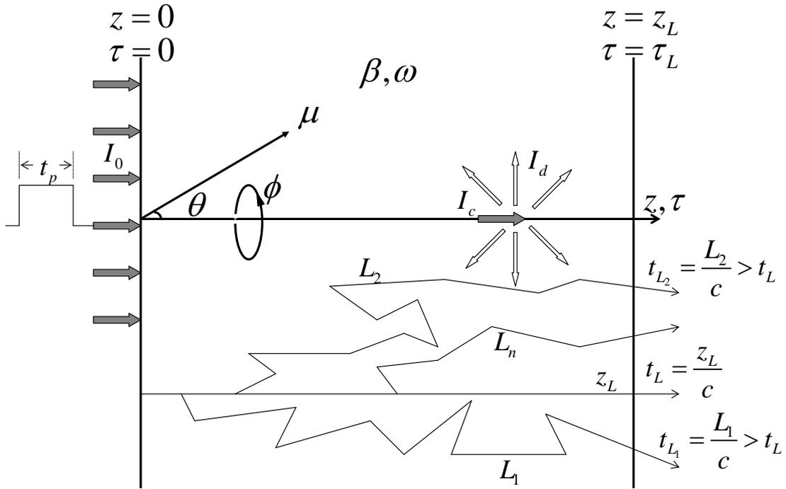
Figure 1: Schematic representation of the transient radiative transfer problem under consideration.
