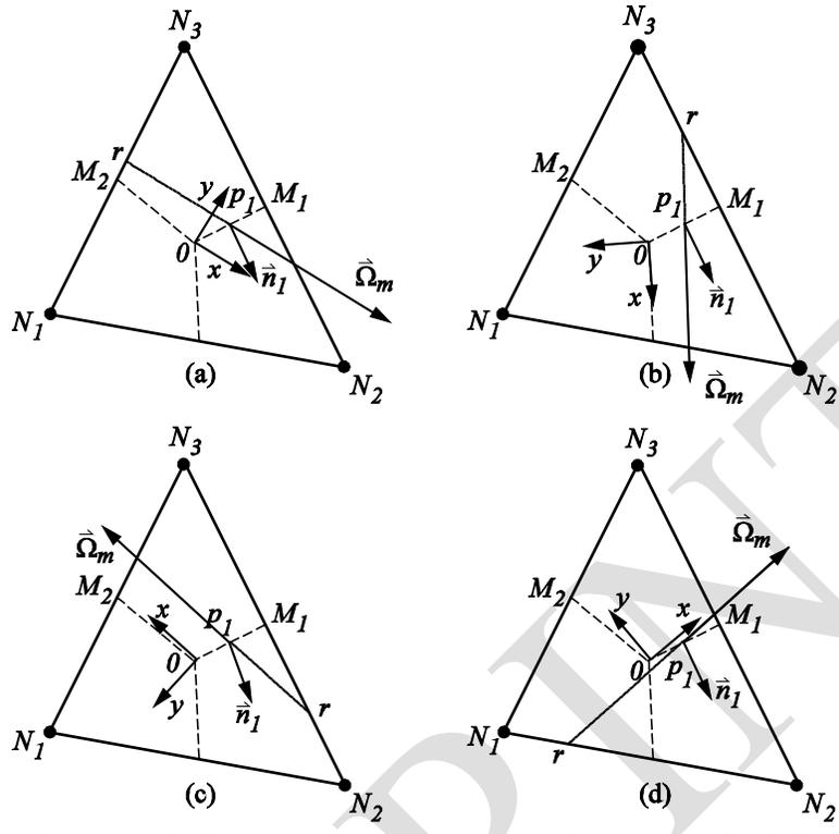
Figure 3. – A basic skew upwind scheme: (a) reference node on edge  $l = 2$  linking  $N_3$  and  $N_1$ ; (b) reference node on edge  $l = 1$  linking  $N_2$  and  $N_3$ ; (c) excellent alignment but reduces to the US; (d) possibility of negative coefficients.
