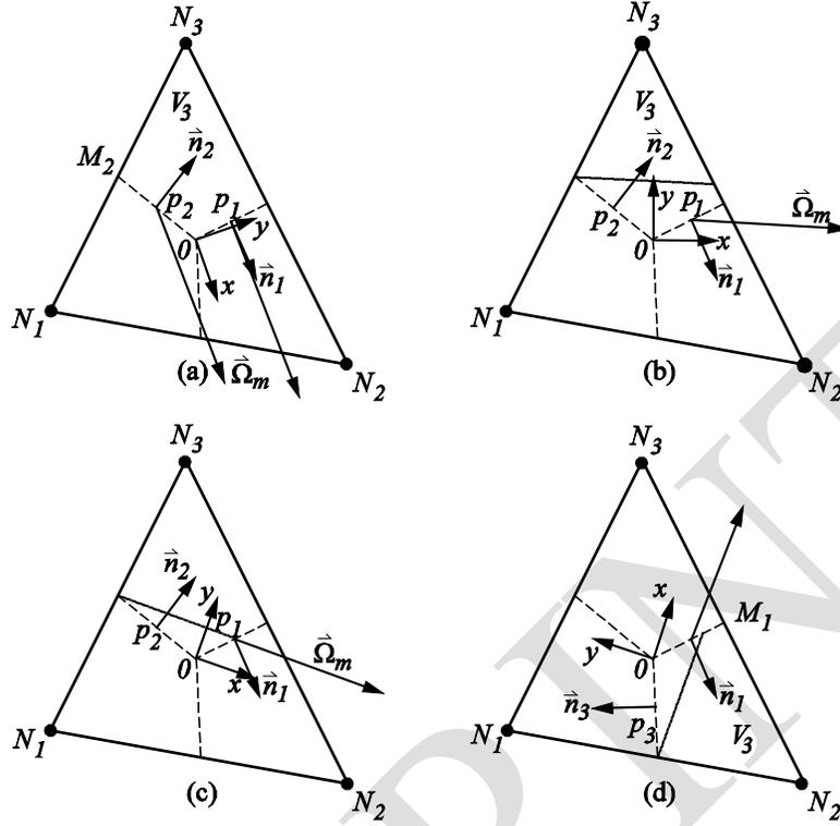
Figure 5. – A skew upwind scheme with positive coefficient: (a) influence of  $N_3$  only when  $y_{M_2} \leq 0$ ; (b) influence of  $p_2$  when  $y_{M_1} \leq y_{M_2}$ ; (c) weighted average of the intensity at nodes  $N_3$  and panel  $p_2$ ; and (d) weighted average of the intensity at nodes  $N_2$  and panels  $p_3$  when  $G_1^m$  is negative.
